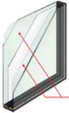
Double Low - E glass (3-10-1.3-10-3) With krypton gas
